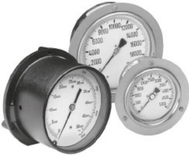
Standard pressure gauges as shown are available from stock for immediate delivery. Gauge models 4PG5 through 6PG50 are standard with a High Pressure  $\frac{1}{4}$ " O.D. tubing connection (HF4), while models 6PG75, 6PG100 and 6PG150 have a Ultra High Pressure  $\frac{3}{8}$ " O.D. tubing connection (XF6). These coned and threaded connections are machined directly into the bottom inlet of the gauges. Adapters for other size connections are available from stock.
